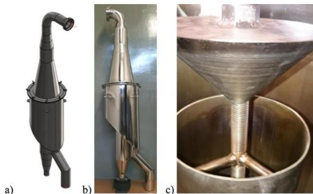
Fig. 3. Inertial-impingement classifier: design (a), fabrication (b), impingement element (c) (courtesy of Promill – cyclone contractor)
