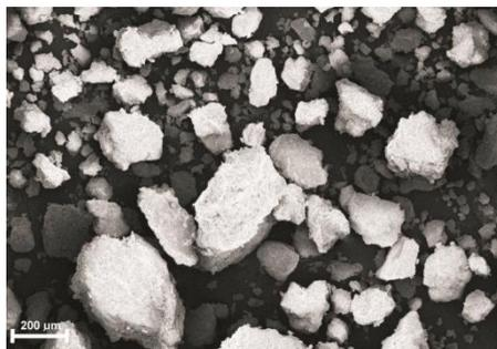
Fig. 4. SEM photo of a raw halloysite from Dunino deposit after milling and 20 minutes of drying
