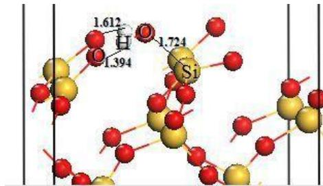
Fig. 9. Optimized adsorption configuration of H<sub>2</sub>O on the quartz surface
